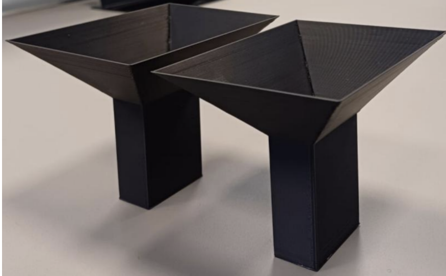
Figure 4.3: Yamacli prototype antenna model manufactured using Protopasta conductive PLA with the identified printing parameters.
