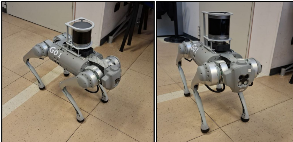
Figure 5.6: Hardware configuration of the Unitree Go1 robot: detail of the RS-Helios LiDAR sensor mounted on the back ( trunk ) inside the protective metal structure.
