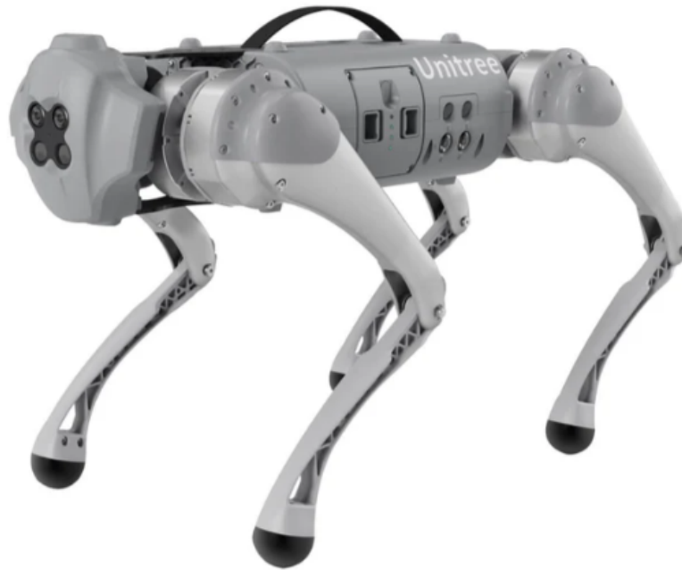
Figure 5.2: The Unitree Go1 quadruped robot selected as the mobile platform for the experimental validation [35].
