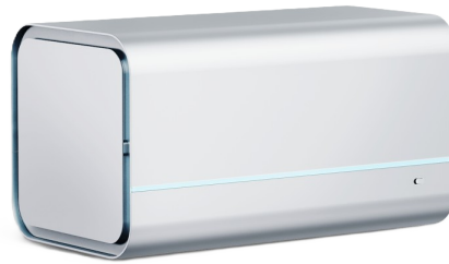
Figure 3.4: The Flexiv HESPER robot controller, responsible for 1 kHz deterministic control loops.
