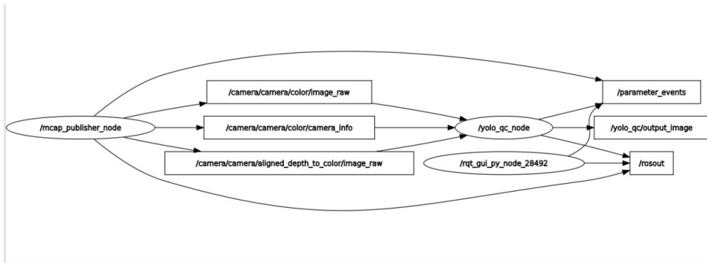
Figure 7.8: rqt_graph representing the pipeline of the program
