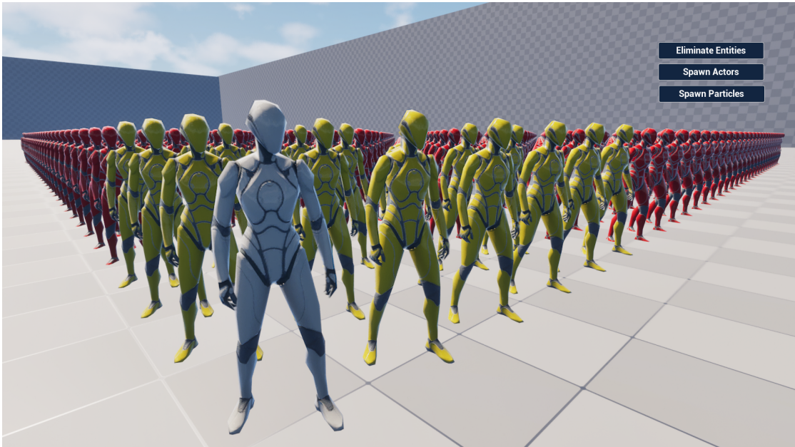
Figure 4.3: Different entity representation based on the distance from the viewer. The red entities are Static Mesh Instances, the yellow ones are LowResSpawnedActors and the white ones are HighResSpawnedActors
