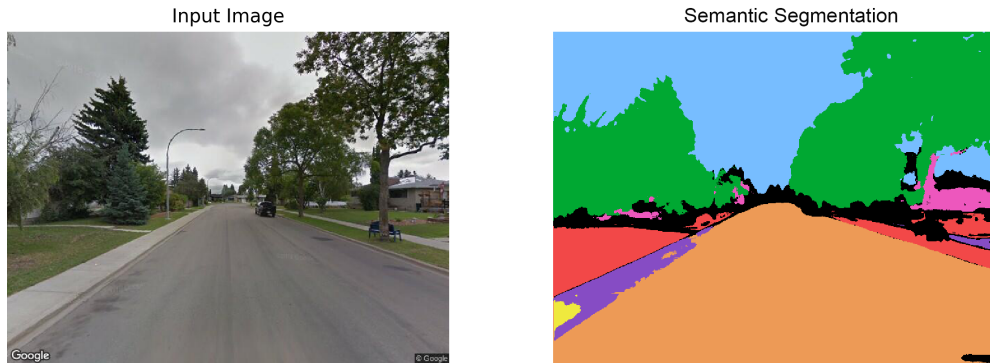
Figure 2.4. Conceptual illustration of semantic segmentation, where each pixel is assigned a semantic class. [16]
