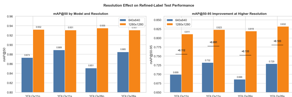
Figure 5.1. Resolution effect on refined-label test performance across all models: left panel shows mAP@50 and right panel shows mAP@50–95, comparing 640 \times 640 and 1280 \times 1280 with per-model improvement annotations.
