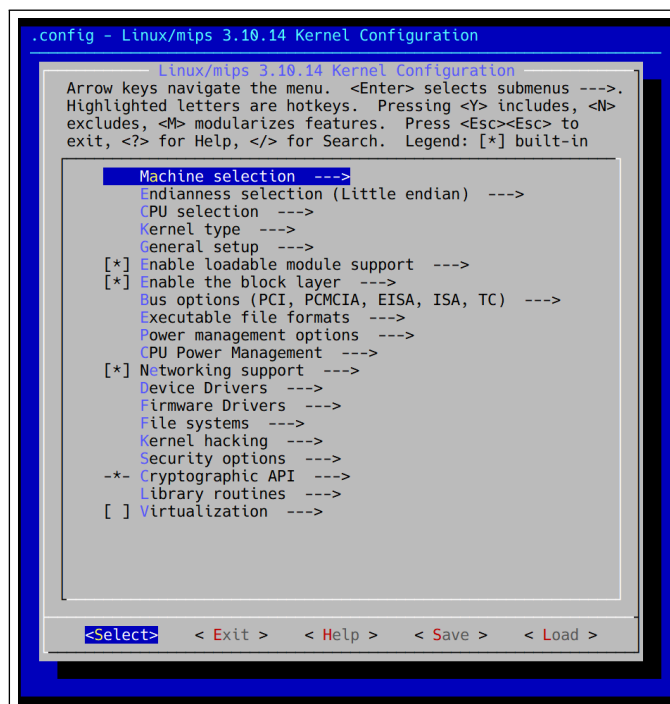
Figure 2.3: menuconfig showing all configurable option categories for Linux. A similar menu exists for Buildroot’s defconfigs .
