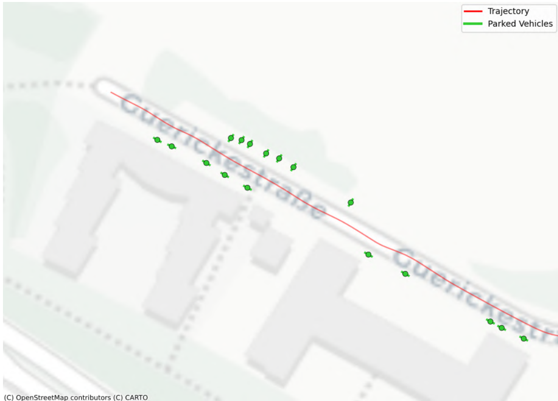
Figure 3.10: Manual refining tool with trajectory and detected parked vehicles displayed over the OSM map
