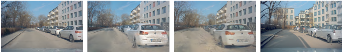
Figure 5.7: Frames generated from the same position by the three techniques compared against the ground truth. Left: ground truth. Center: 3DGS and NeRF, which exhibit perspective misalignment due to trajectory replay errors. Right: Stable Diffusion, whose perspective more closely resembles the real-world viewpoint thanks to its conditioning on semantic segmentation maps.
