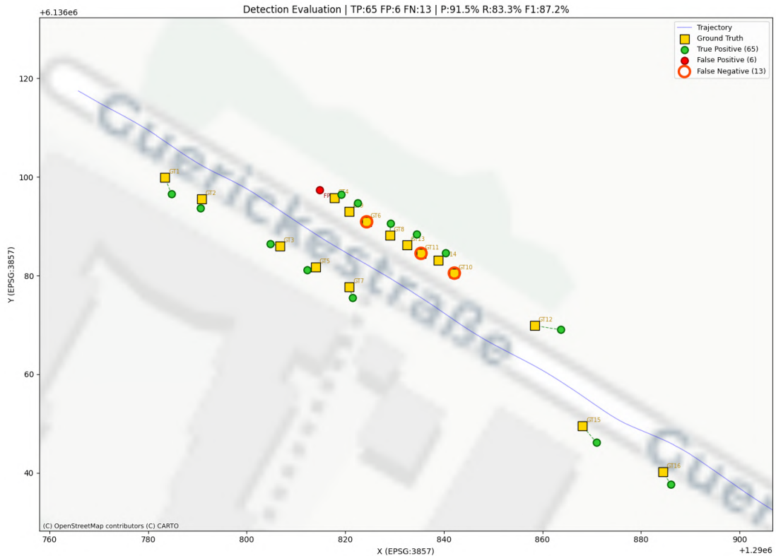
Figure 4.15: Example of predicted vehicle positions and ground-truth annotations overlaid on an OSM map. Green dots indicate correctly matched vehicle detections, while red dots indicate detections that could not be associated with any ground-truth vehicle and are therefore counted as false positives. Yellow squares represent ground-truth vehicle positions; those highlighted with a red circle indicate false negatives.
