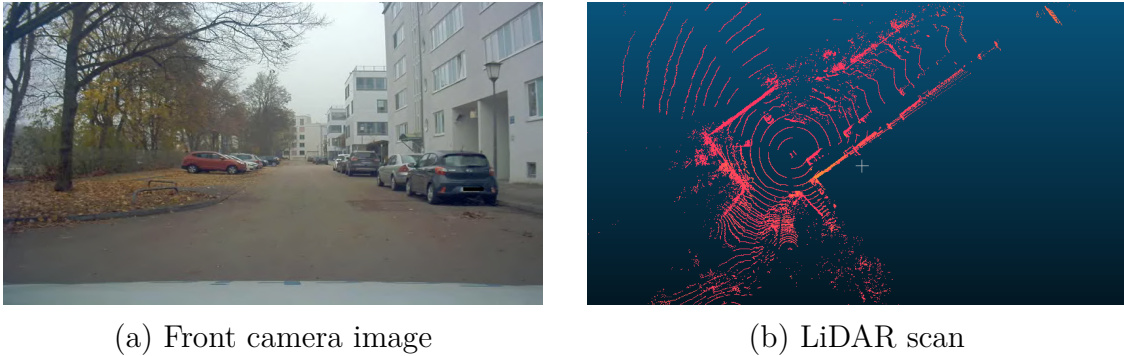
Figure 3.3: Example of a front camera image and the corresponding LiDAR point cloud recorded by the ego vehicle.
