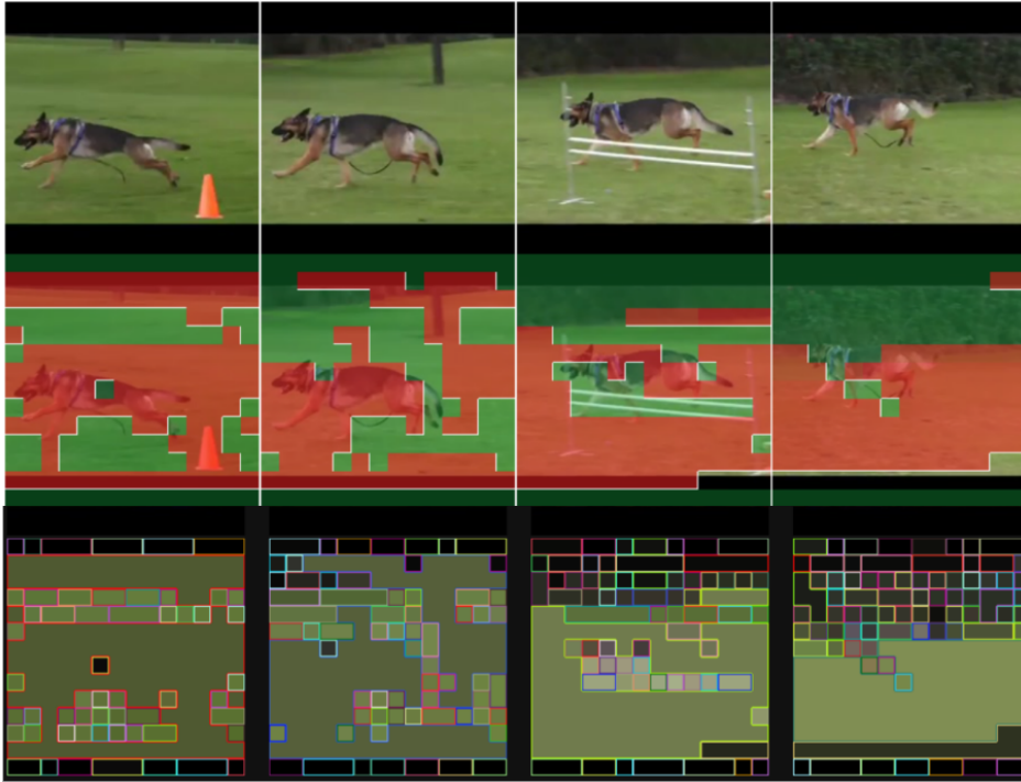
Figure 5.8. Qualitative visualization of the TBKV pipeline on a video from the Kinetics-400 dataset labeled training dog . The first row shows consecutive frames from the video sequence. The second row illustrates the saliency-based foreground/background separation, where foreground tokens are highlighted in red and background tokens in green. Dynamic regions corresponding to the dog and nearby interaction areas are correctly identified as foreground, while static regions such as the grass field, image borders, and distant scene elements are classified as background. The third row visualizes the merging of background tokens during the cache warm-up phase. Colored rectangles represent groups of tokens that are merged using bipartite soft matching, forming compact background representations that are stored in the cache. Large uniform regions are aggressively merged due to their high redundancy, while areas near the moving subject preserve finer token granularity.
