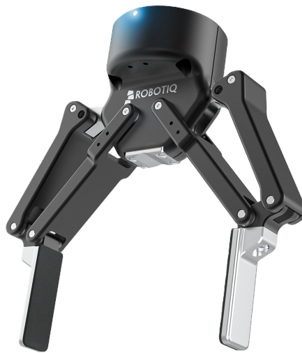
Figure 3.2: Robotiq 2F-140 gripper (taken from [27])
