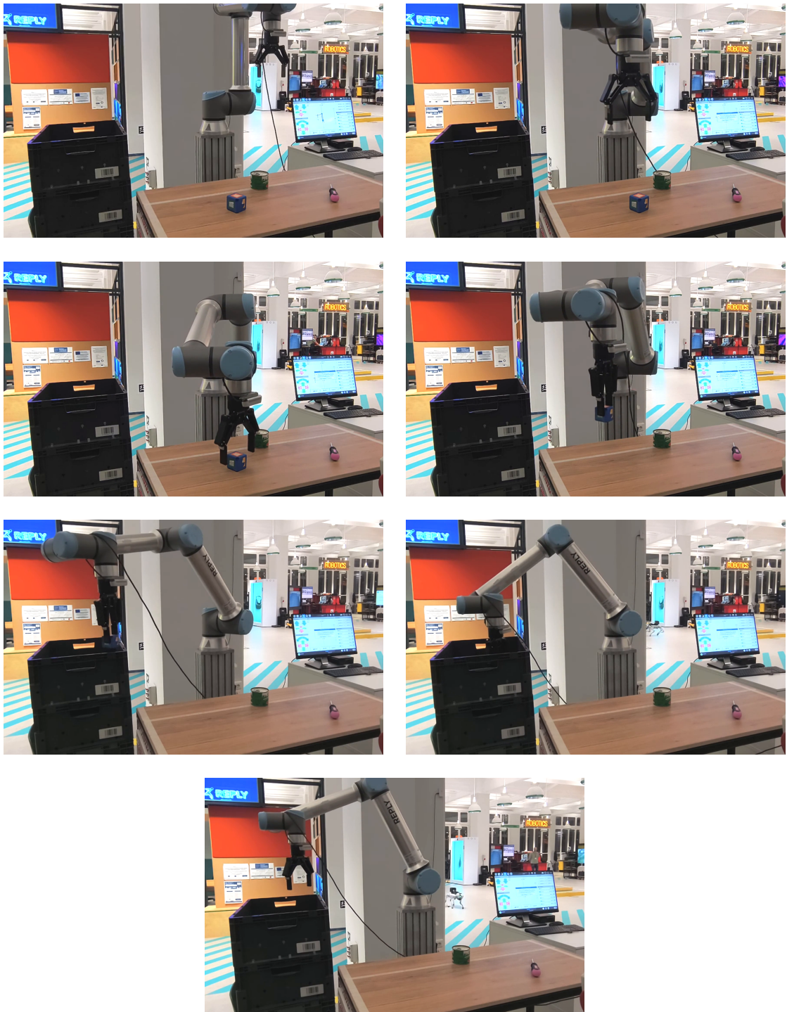
Figure 6.2: Pick-and-place: Key frames from full real-world task demonstration
