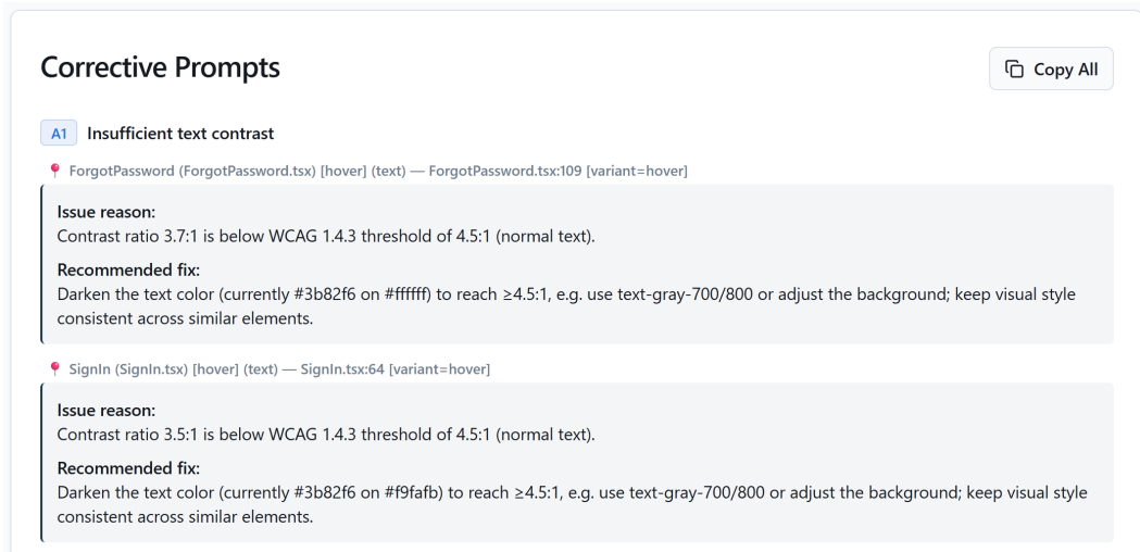
Figure 4.7: Example corrective prompt generated for rule A1 (Insufficient Text Contrast), including the detected issue and recommended fix.
