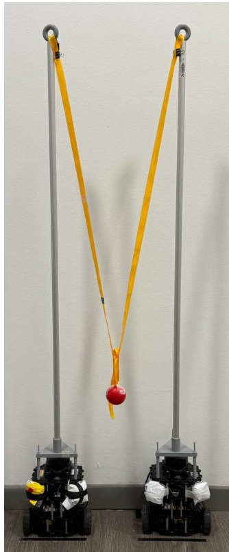
Figure 2.1: Experimental setup for cooperative transport with rope-based coupling.
