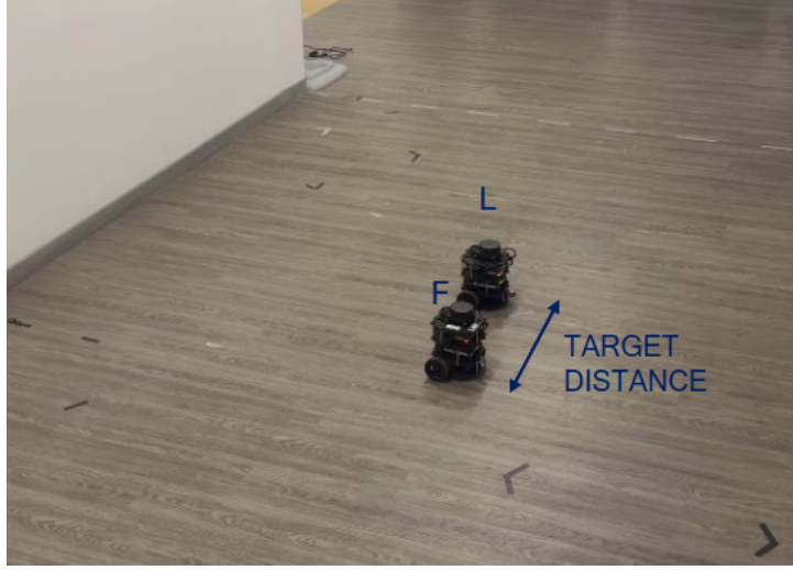
Figure 5.2: Left-lateral configuration: the follower tracks a goal point at distance d along \mathbf{n}_L
