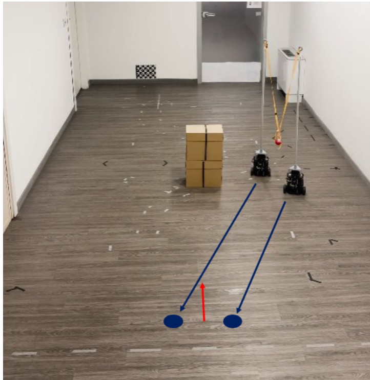
Figure 6.2: SETUP phase: the robots move from their initial positions to the formation configuration defined by the virtual centre. Blue arrows indicate the commanded trajectories; the red arrow represents the virtual centre position and heading.
