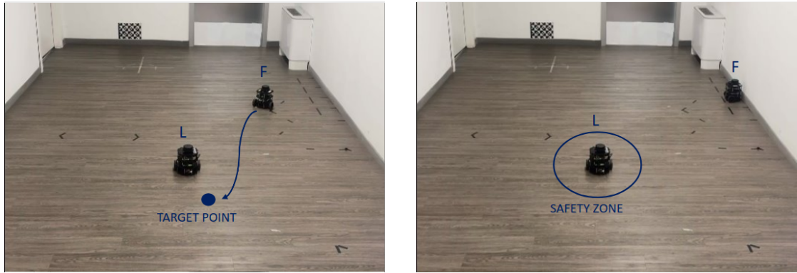
(a) Path generated by the controller towards the formation target point (b) Safety zone (no-go disc) around the leader
