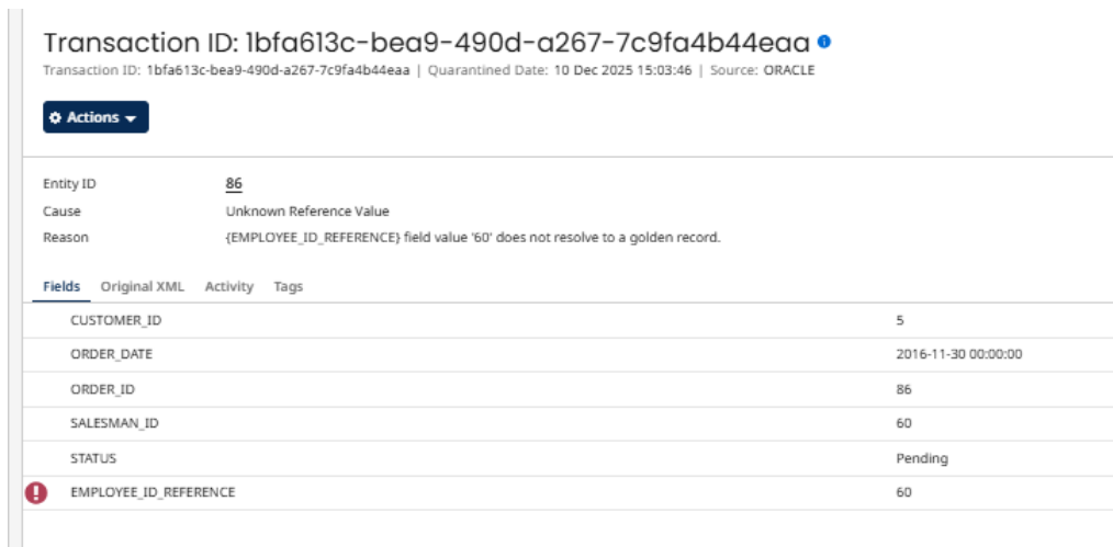
Figure 8.23: Detailed information on the quarantined record and the reason for the quarantine, namely the EMPLOYEE_ID referential integrity
