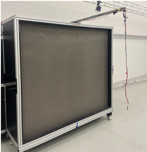
(c) WindShape wind tunnel for hover tests
