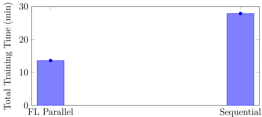
Figure 6.4: Total training time comparison: Federated (parallel) vs. sequential per-client training.
