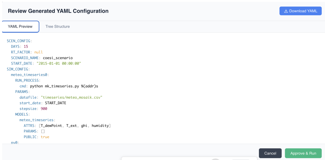
Figure 6.7. YAML review modal shown after compilation: the generated configuration can be inspected (and optionally copied/downloaded) before it is uploaded and executed.
