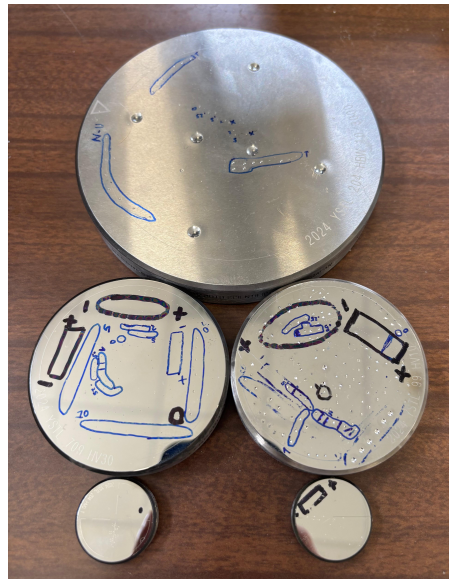
Figure 3.10: Certified reference blocks used in the experimental campaign. From top to bottom: Brinell block, macro-Vickers blocks and micro-hardness blocks used for Vickers and Knoop measurements
