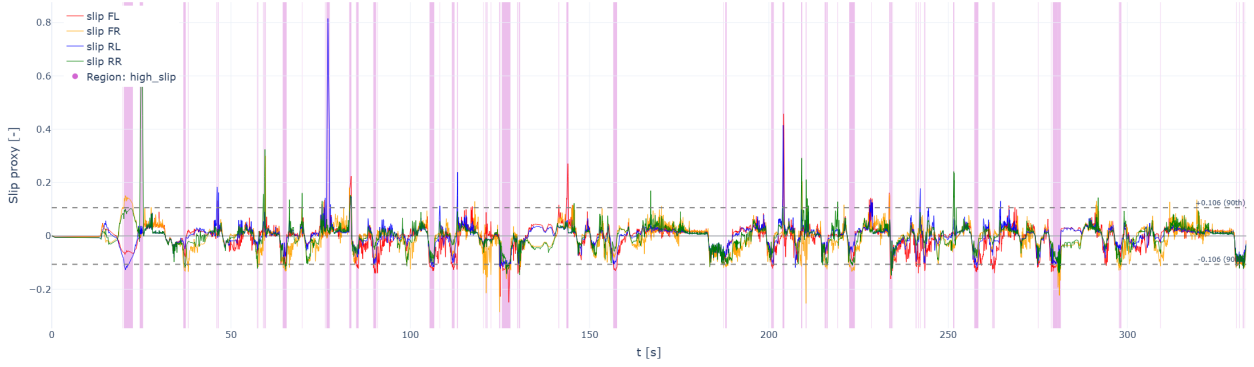
Figure 8.3: Slip proxy signals and identified high-slip conditions for the test run.
