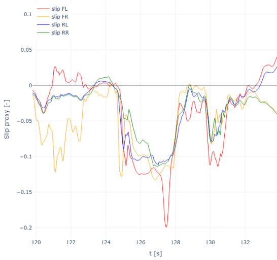
(a) Wheel slip during the multi-wheel slip event. All wheels exceed the high-slip threshold.
