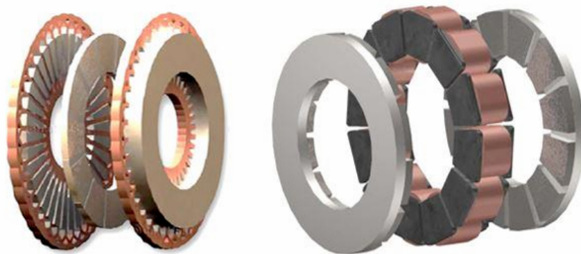
Figure 2.7: Structure with double stator (on the left) and with double rotor
