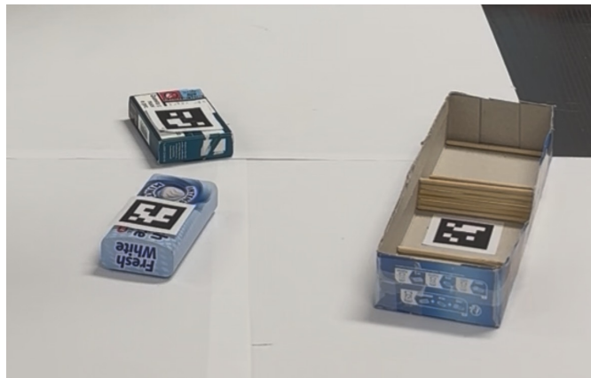
Figure 4.9: Example of ArUco Markers placed on different objects
