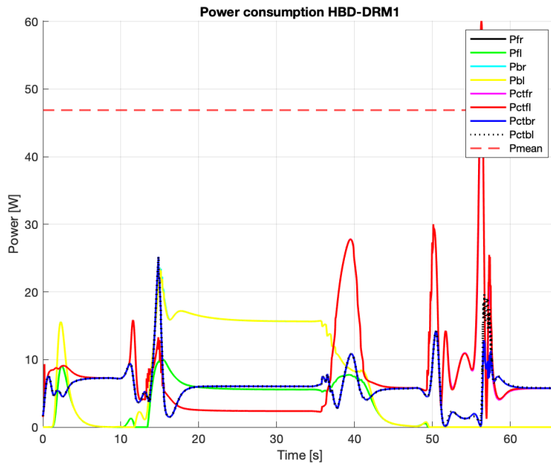
Figure 7.13: HBD power consumption
