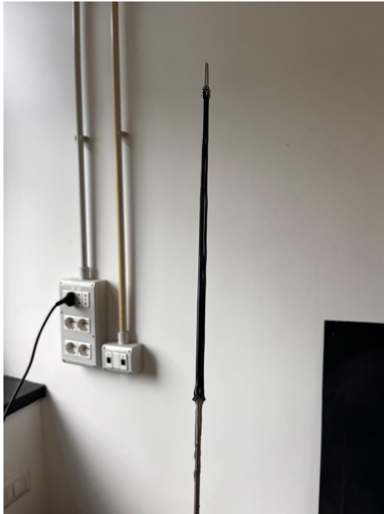
Figura 3.5: Prototype of the first model: braided sleeve (fiber 187-4600) pre-coated with silicone and supported by a thin metal tube during fabrication.
