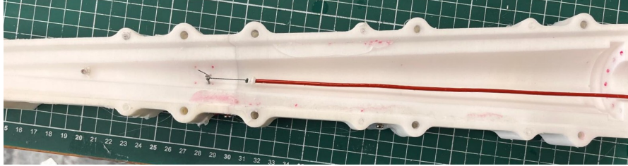
Figure 3.18: Fourth design prototype integrating a silicone-rubber-coated braided fiberglass sleeve as internal reinforcement.
