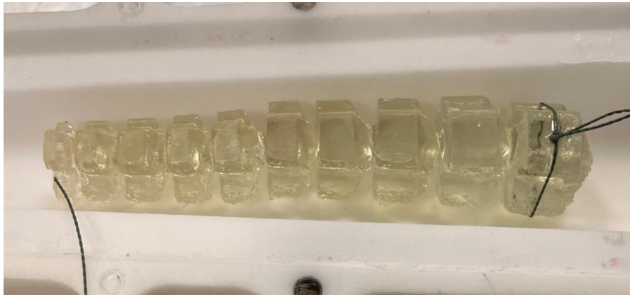
Figura 3.21: Resin-printed prototype of the reference SpiRobs-inspired geometry, cast in silicone to qualitatively assess resin–silicone adhesion and bending behaviour.
