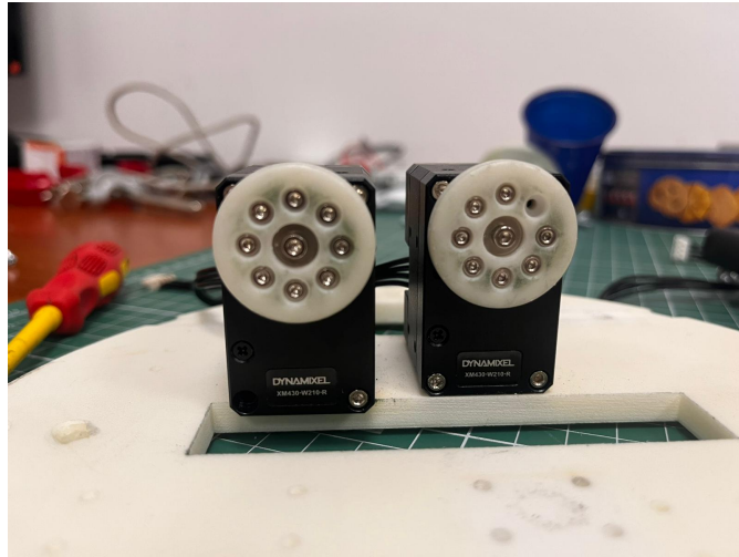
Figura 4.1: Dynamixel XM430-W210-R servo motors used for tendon actuation.
