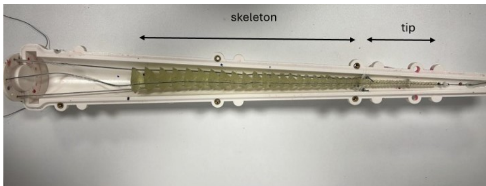
Figure 3.30: Internal assembly of the final prototype before silicone casting: the previously developed internal skeleton is integrated with the tooth-like distal tip, while the nylon fishing line is routed through a protective sleeve and anchored proximally via a dedicated support.
