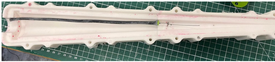
Figura 3.14: Mold with the fiber insert
