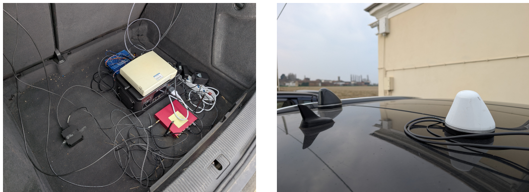
Figure 6.1: Experimental setup installed on a moving vehicle.
