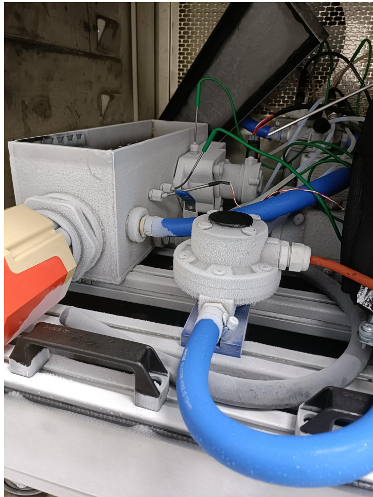
Figure 7.1. Conditions of the rig after reaching T = -40^{\circ}\text{C} without the EOP running.
