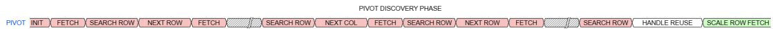
Figure 3.11: Example timing the pivot discovery phase, highlighting row scanning and pivot selection. The timing is illustrative; internal state lengths are not exact.
