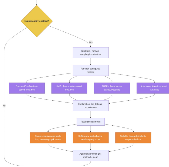
Figure 6.4: Flowchart detailing the Explainability Orchestrator phase.
