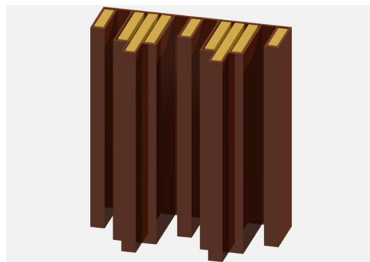
Figure 4.2 The rendering illustrates the Schroeder diffuser as it would appear under examination, with the internal filling clearly delineated in the sectioned top.
