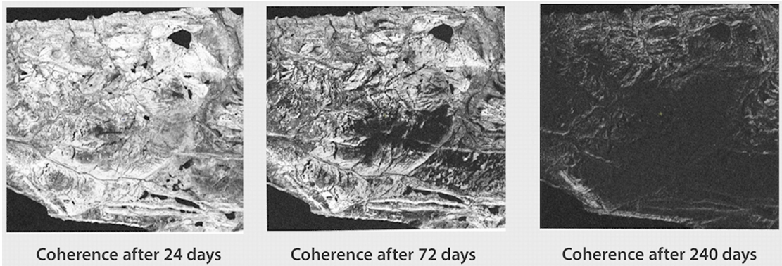
Figure 3.2: Degradation of coherence over different temporal baselines. Areas become darker as scattering properties change over time, [26].
