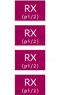
Figure 1.6: This figure illustrates the Mixer Unitary for a system composed of four qubits [22]. Also here the parameters to optimize are randomly set to \frac{\pi}{2} .
