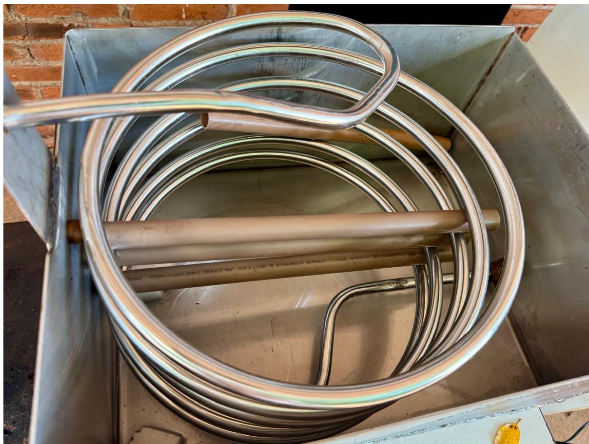
Figure 3.6: Heat Exchanger. Credit: Author
