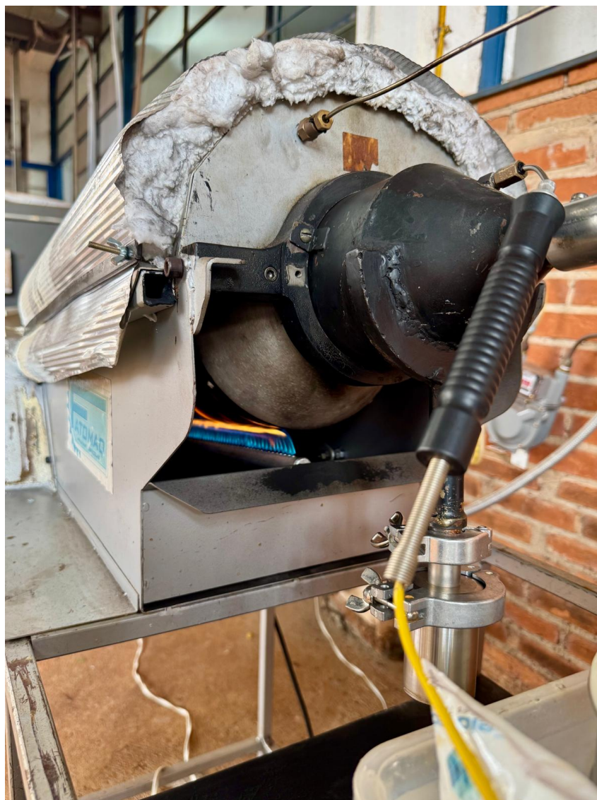
Figure 3.5: Funnel at the reactor outlet with a compartment for bio-oil collection. Credit: Author
