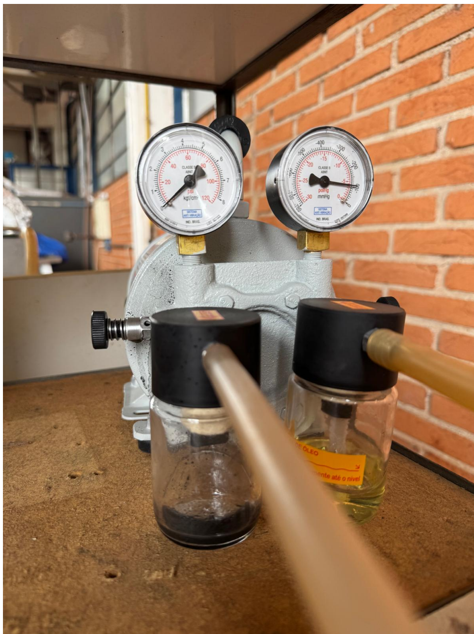
Figure 3.9: Vacuum Pump. Credit: Author
