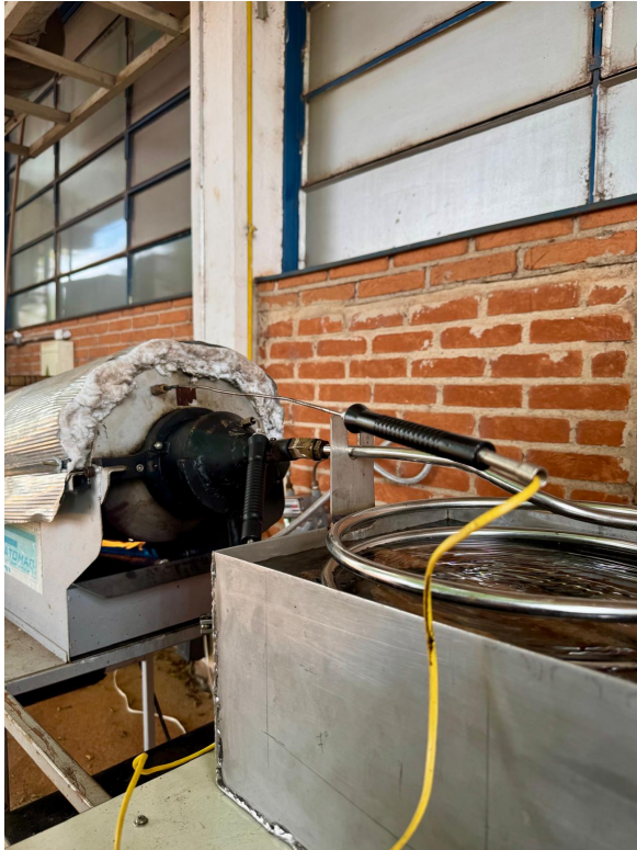
(a) Reactor and condensation coil used during the pyrolysis experiment. Credit: Author
