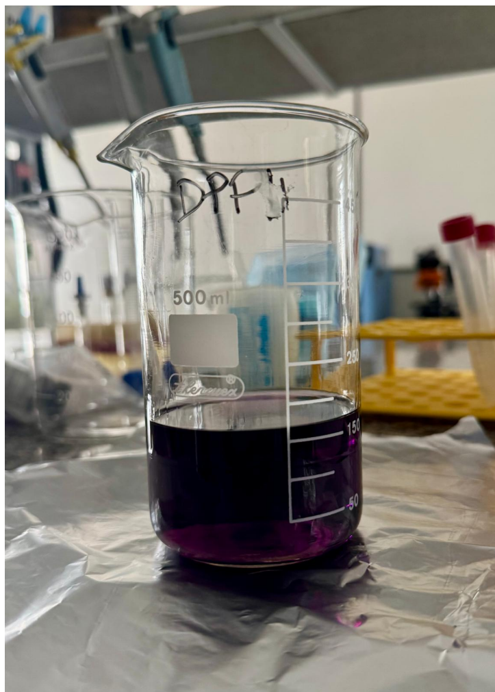
Figure 3.14: Beaker containing the freshly prepared DPPH solution prior to light protection with aluminium foil. Credit: Author
