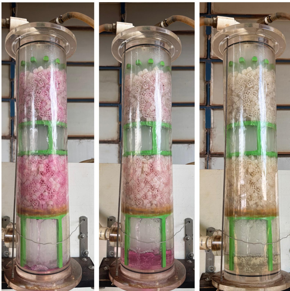
Figure 3.8: Gas-scrubbing column showing the three color states observable during the experiment: basic (pink), neutral (light pink), and acidic(colorless).Credit: Author
