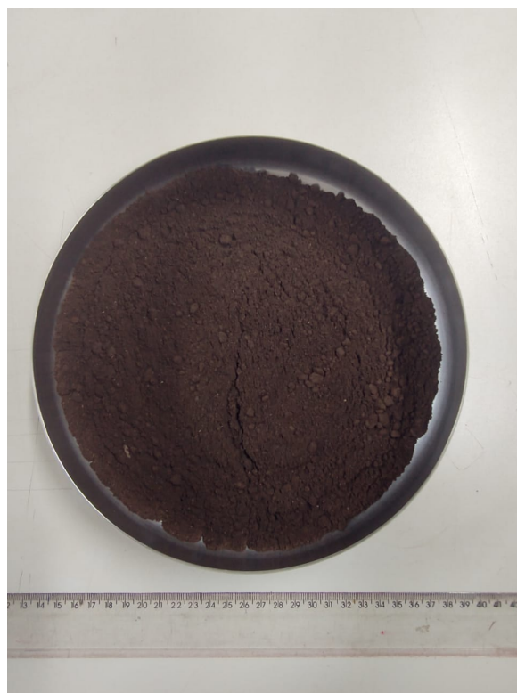
(b) Dried SCG after 24 h of oven drying at 100 °C. Credit: Author
