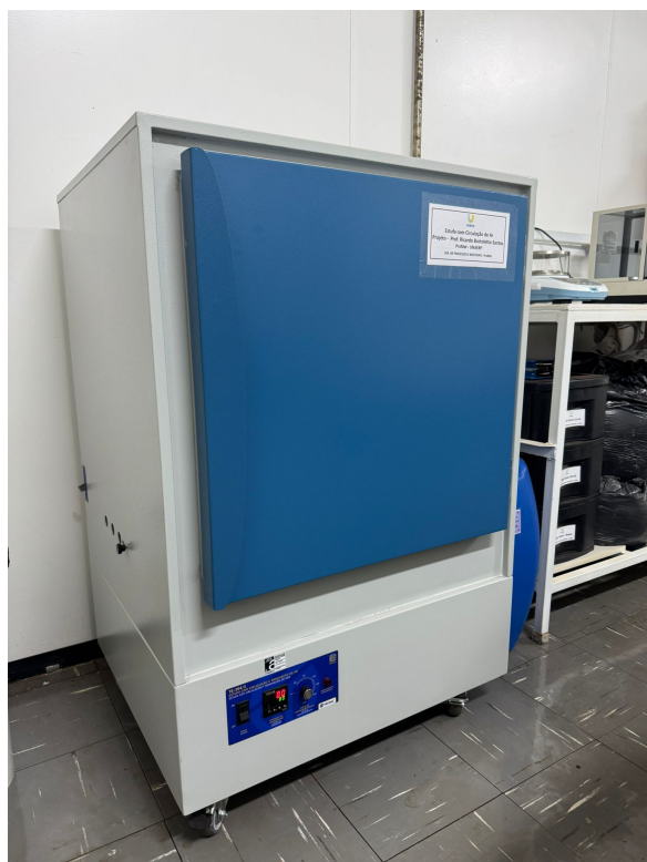
(a) Oven used for drying the SCG prior to pyrolysis. Credit: Author
