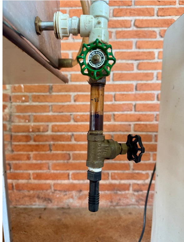
(b) Transparent drain tube equipped with two valves for bio-oil collection. Credit: Author
