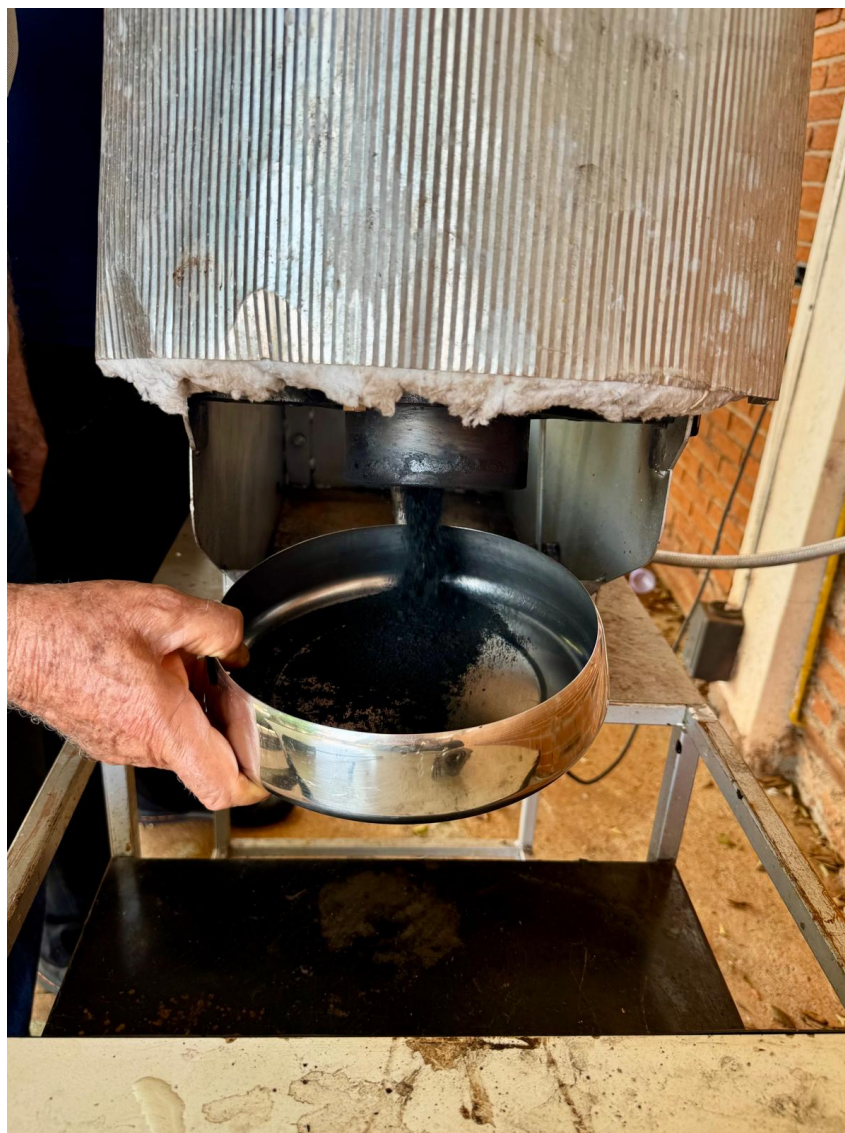
Figure 3.11: Manual collection of the biochar after the cooling phase of the reactor. Credit: Author
