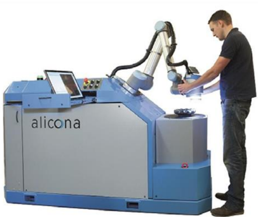
Figure 21: Collaborative robot, equipped with a high-resolution 3D sensor [47].
