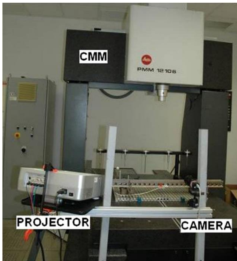
Figure 20: Representation of a hybrid system [45].
