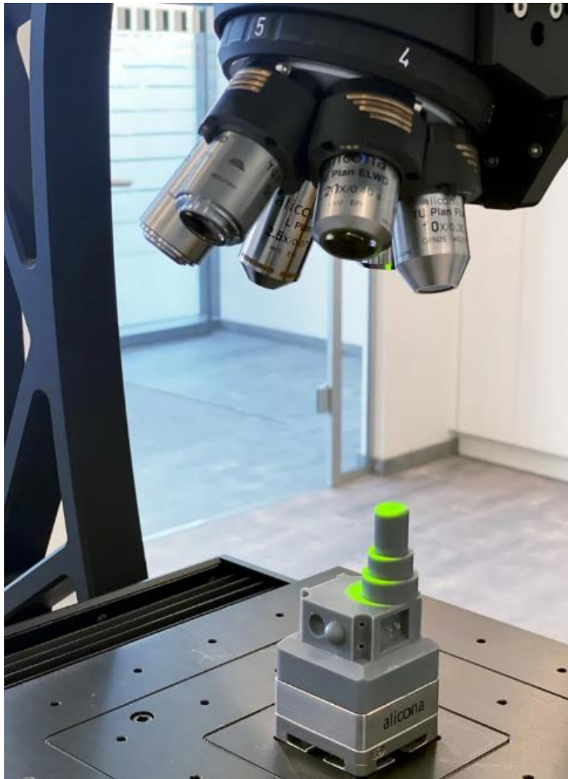
Figure 17: Precision optics for focus variation technique [37].
