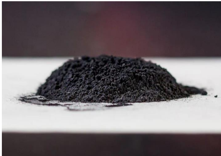
Fig. 2: Black mass obtained from mechanical processing of spent lithium-ion batteries. Source: ISPI.
