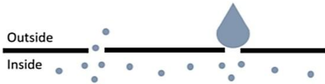
Figure 4 - Hydrophilic porous membrane [1]
