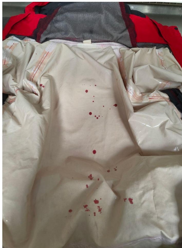
Figure 16 - Effects of IPA on micro holes in the membrane
