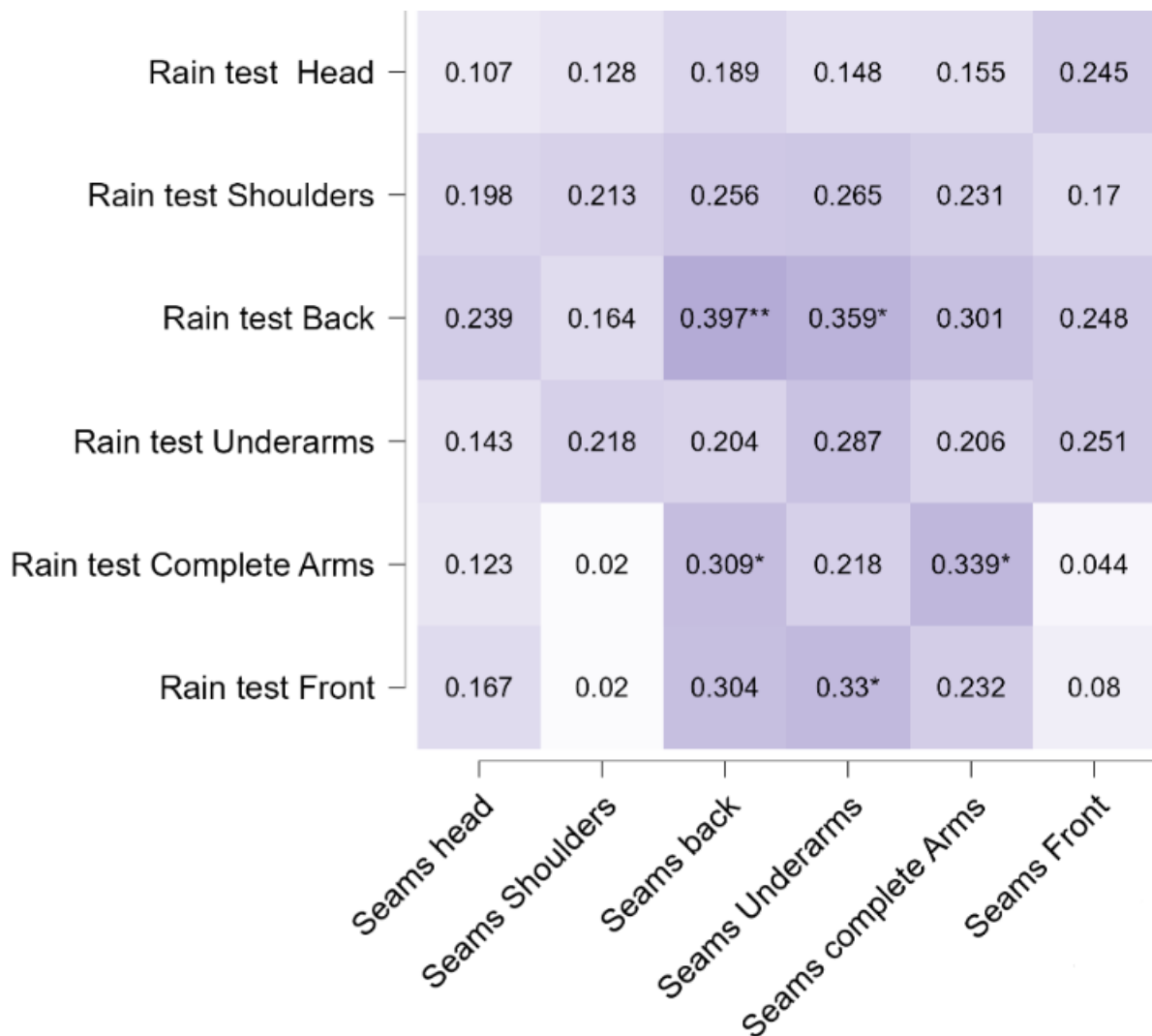
Figure 14 - Heat map for the correlation between the rain test and the seams
