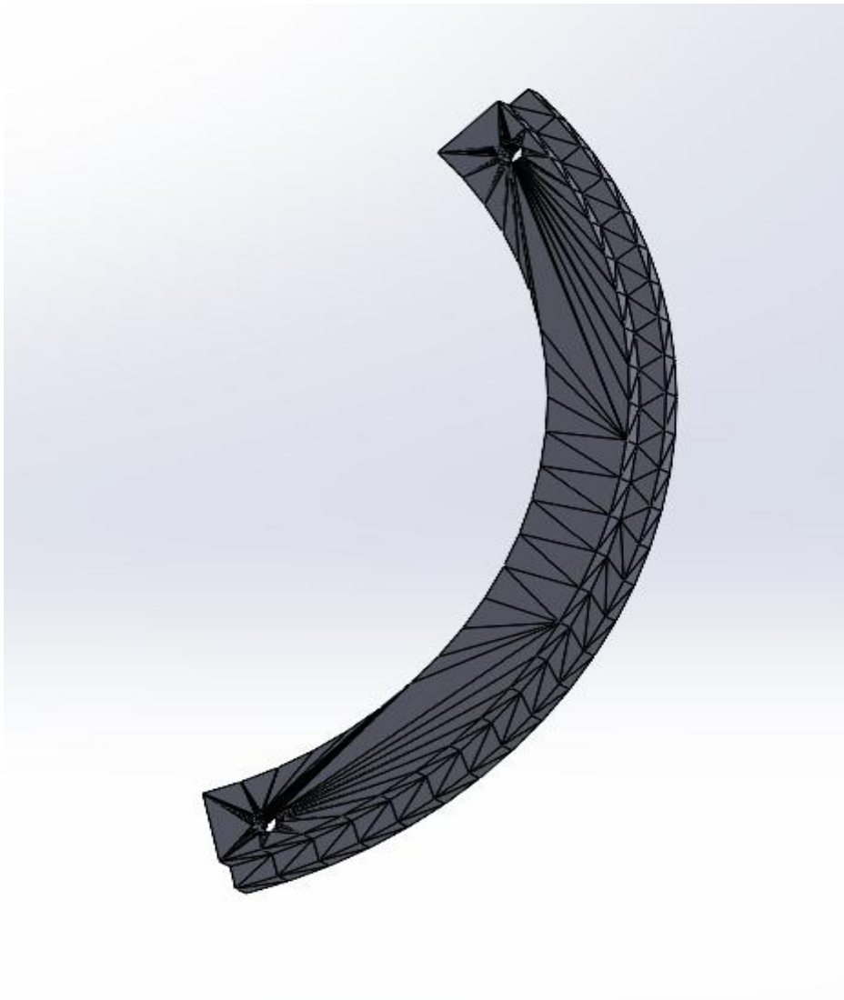
Figure 2 : Felt seal holder, designed with SolidWorks and 3D printed with PTEG
