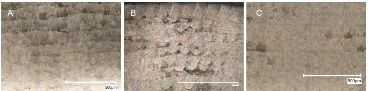
Figure 20 : Optical microstructures of samples fabricated under continuous ultrasonic vibration applied to all layers in intermediate mode with a 5 s stabilization period prior to scanning (Samples 4–6). The micrographs correspond to specimens located at different distances from the ultrasonic source: (a) near the center of the substrate plate, (b) intermediate distance, and (c) farthest distance. Overlapping melt pool boundaries characteristic of the layer-by-layer process are visible across the microstructure.
