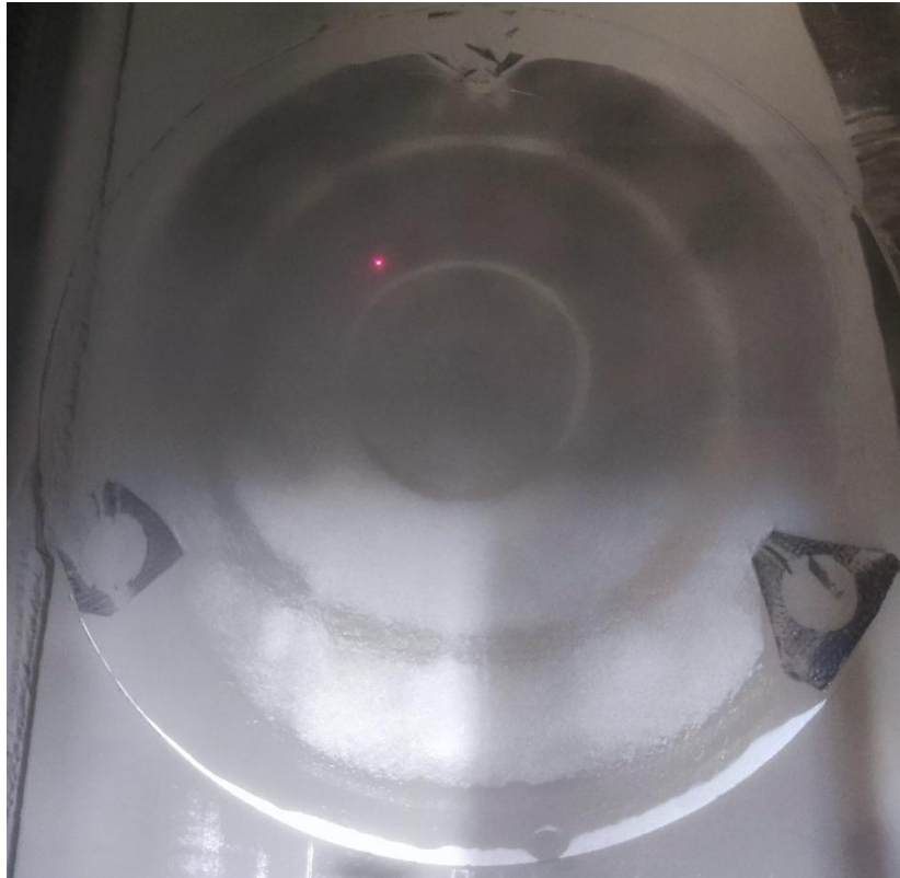
Figure 8: Chladni plate pattern for 70 khz sonotrode on c45 base plate.
