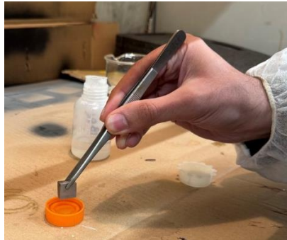
Figure 14. Etching process of the samples with Kroll etchant.
