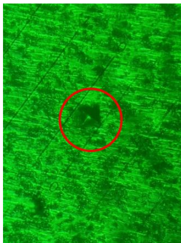
Figure 16. Impact of diamond indenter on the surface of the sample.
