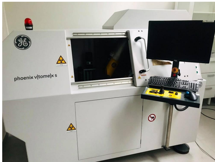
Figure 11. Phoenix v|tome|x s CT machine with integrated interface.
