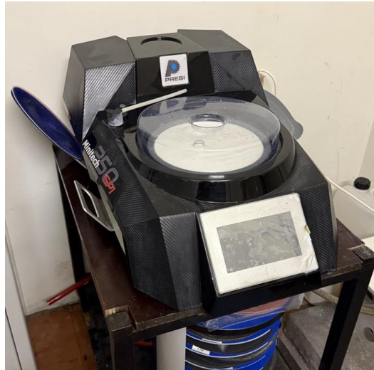
Figure 13. Presi Mini tech 250/300 SP1 grinding machine.
