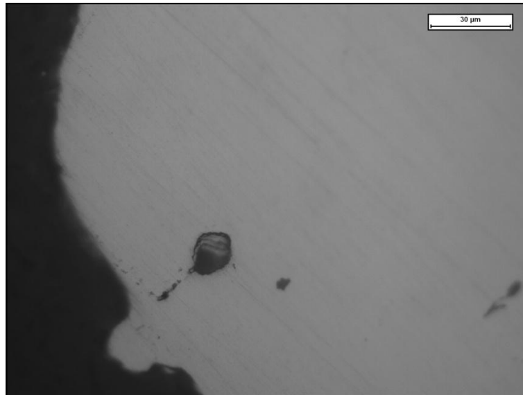
Figure 3.5: Optical micrograph of open porosity near the surface of a HIP-processed sample.
