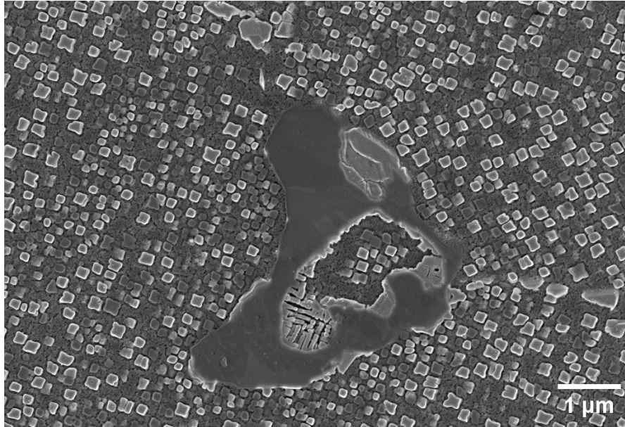
Figure 3.35: Detailed SE image of a large mixed carbide.
