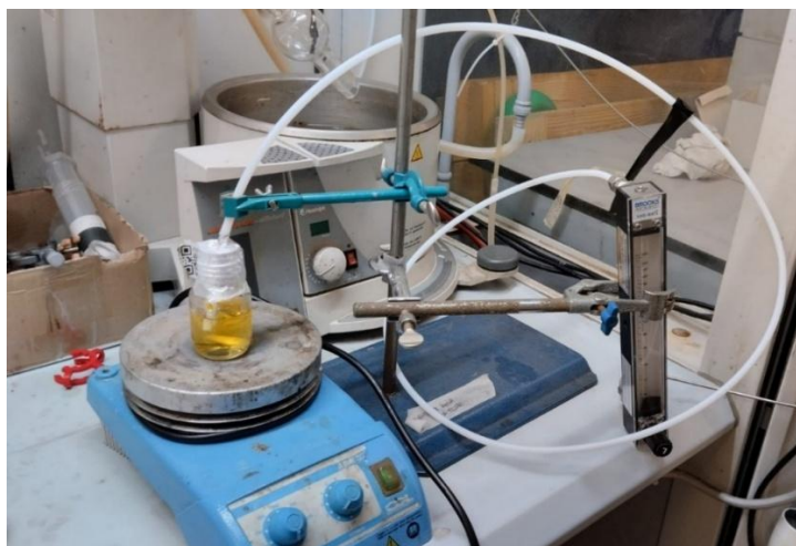
Figure 2.2. Reaction system for system and heating of the solution of Chloroplatinic Acid Hexahydrate, NaOH and EG for Pt nanoparticles synthesis.
