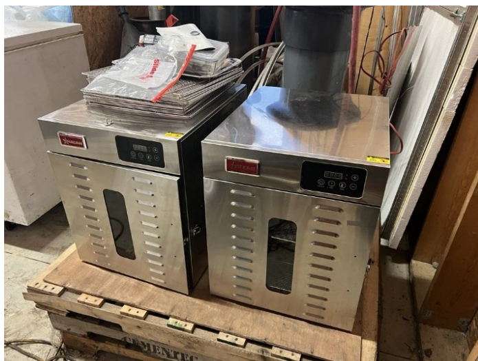
Figure 6.2: Laboratory oven used for air-drying of biosolid samples
