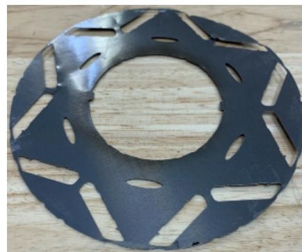
(b) Rotor lamination. [2]
