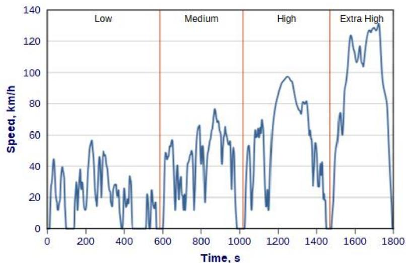
**Figure 2.3.** WLTP cycle for Class 3b vehicles [39].
