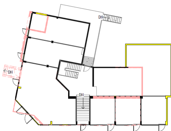
⬆ Fig.19 and Fig.20 - Ground floor of Honigmann House from from ca. 1930 (on the left) and 1937 (on the right), demonstrating the assumed demolition (in red) and new construction (in yellow)relatively to the previous phase of the building (for scaled version and rest of the comparative plans see fig.A.6 and fig.A.7 in appendix). Source: drawings by the author.
