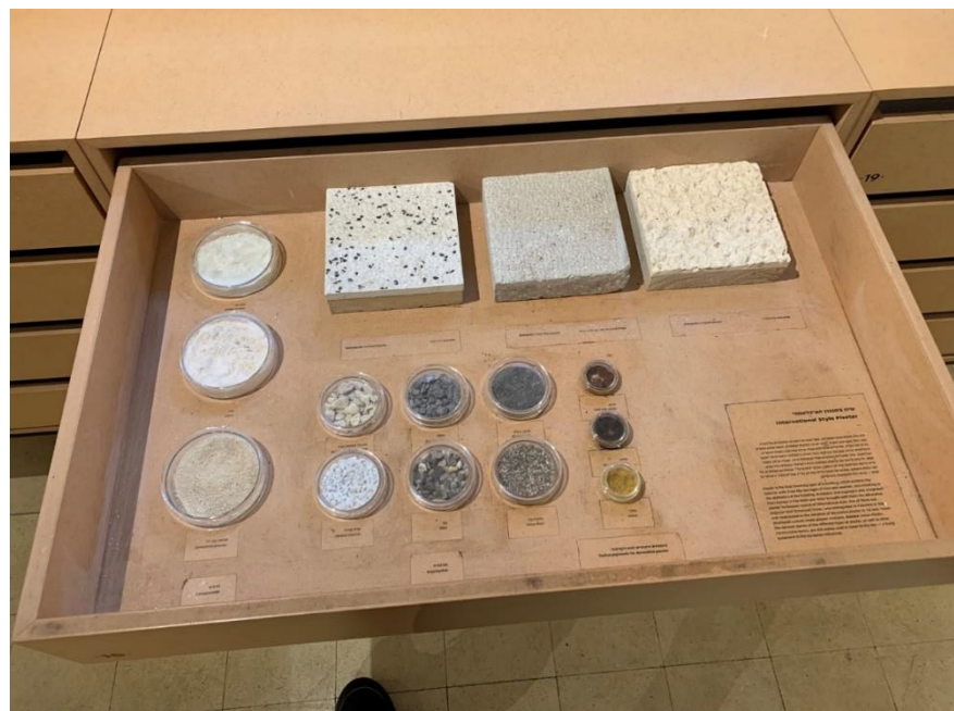
Fig.23 - Samples of different typologies of plasters in various solid forms, used in international style buildings (including Liebling Haus). Source: photo by the author. August 26, 2024.
