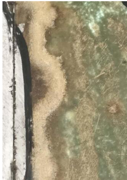
fig. 16. Exposed glass-fibres in a GRP shell, with white chalking visible. Image Pizzigati & Franzoni 2021.
