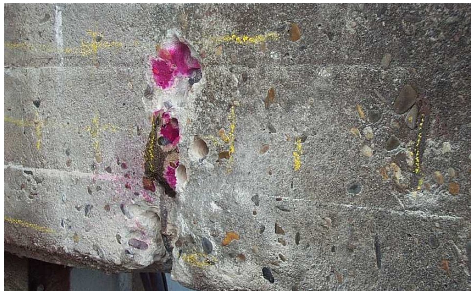
fig. 22. Testing of carbonatation depth by phenolphthalein. The purple parts are not carbonated. Photo C. van der Steen, Technoconsult Heeswijk.
