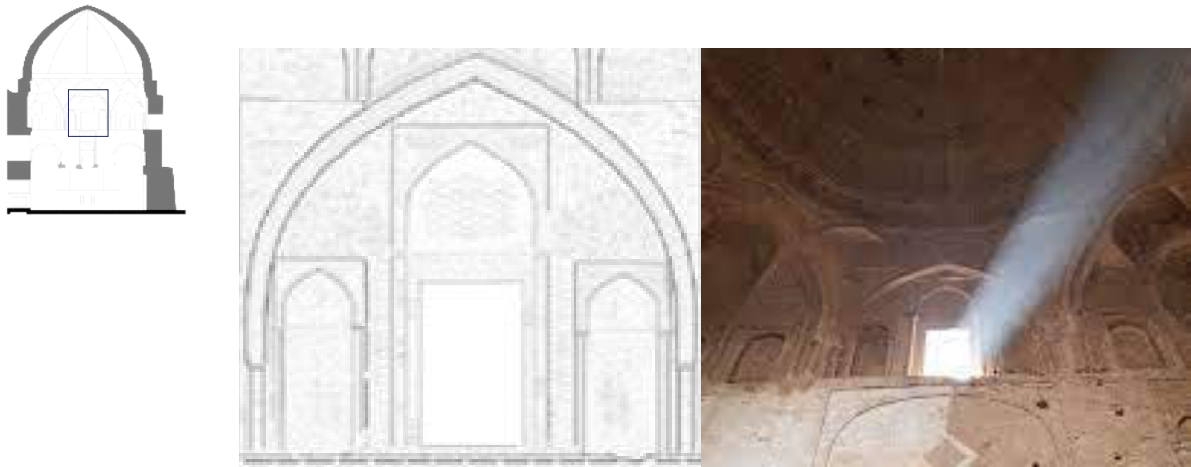
Fig. 112 the openings of transition zone Nezam al-Molk Dome, reference: personal archive.
