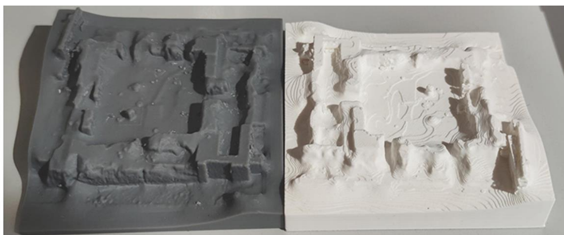
Fig. 67 Comparison of preliminary test FDM and VPP printed models
