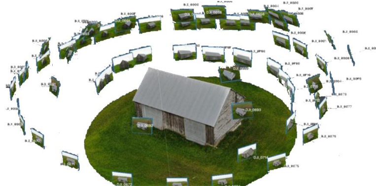
Fig. 24 Photogrammetry based on photo modeling provides high-overlap-rate photos from multiple angles, and uses algorithms to capture key point matching to generate models.
