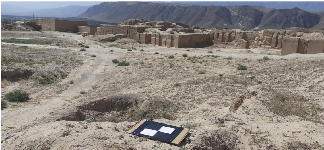
Fig. 19 Checkerboard targets used for on-site measurement point positioning
