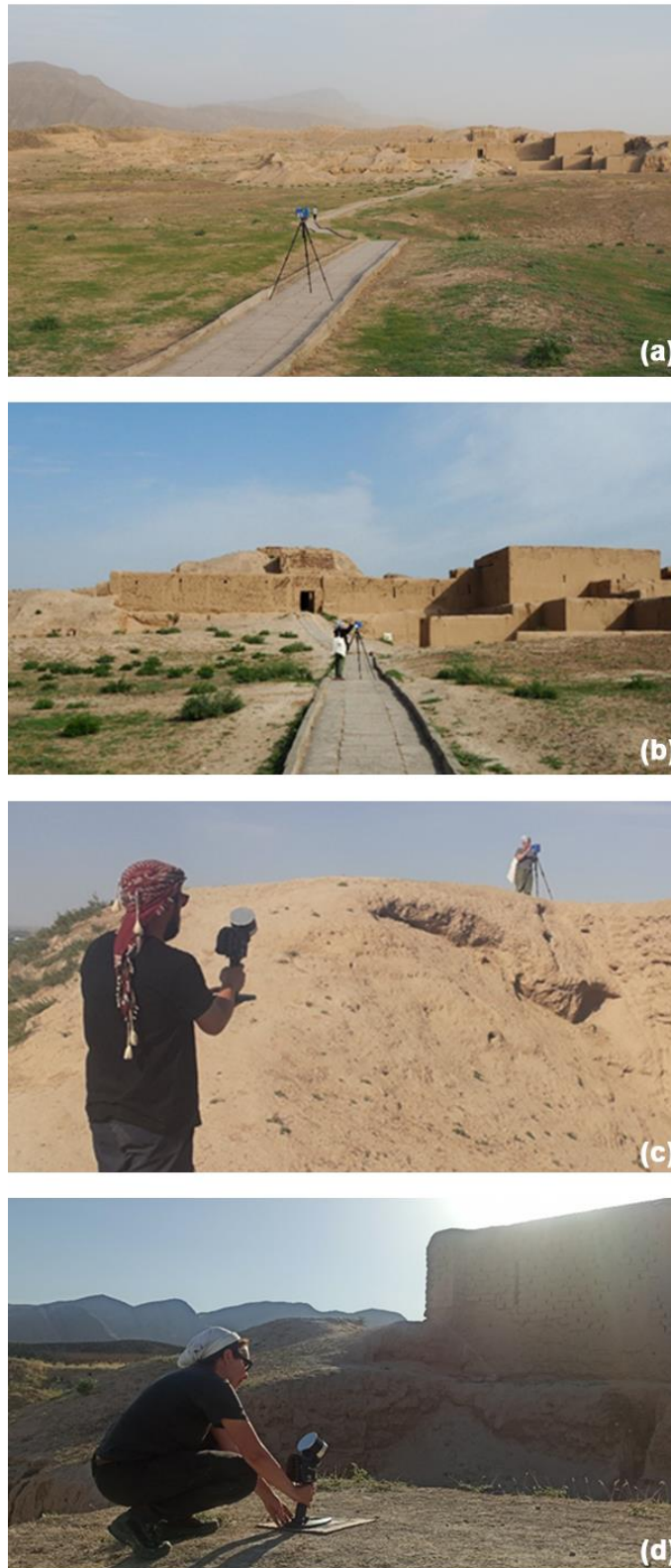
Fig. 25 (a)(b) TLS scanning operation (c) SLAM and TLS scanning operation (d) SLAM at checkpoints
