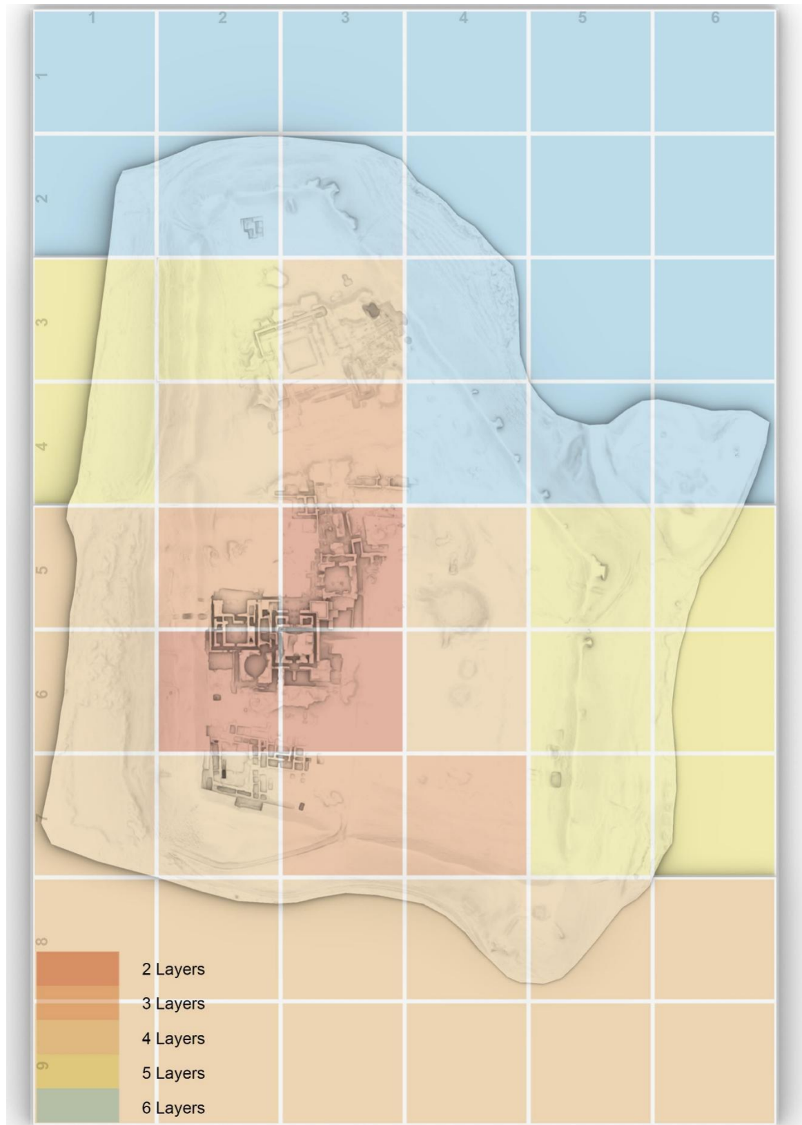
Fig. 70 Number of layers of the wooden support base determined based on the zoning
