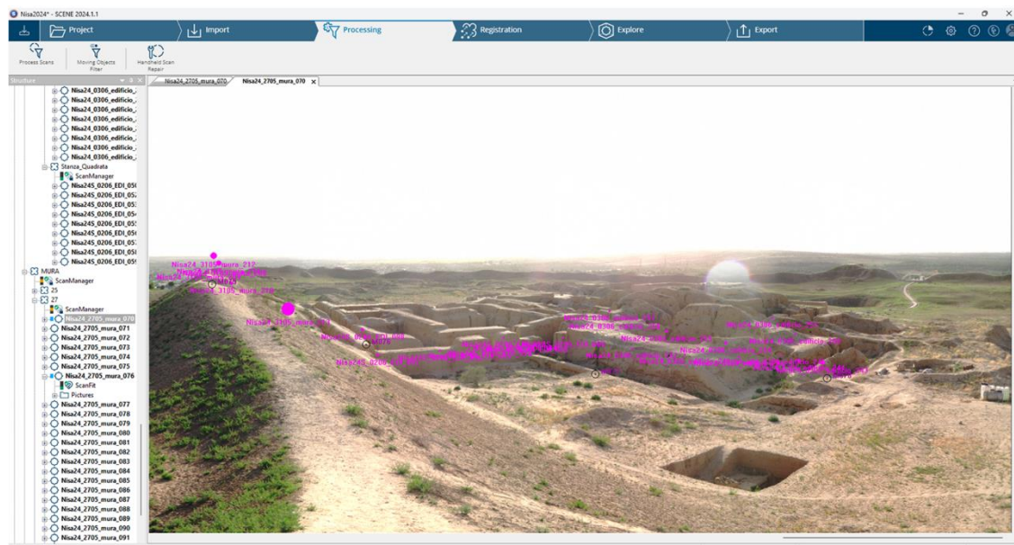
Fig. 31 Mura 27 slice as example, the scanned point cloud and image are integrated into the scene, and the scanned points within a sub-file are visible
