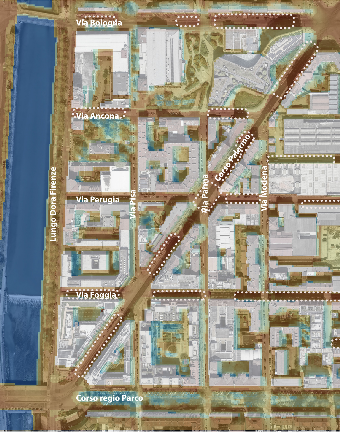
Fig. 107 Identifying the most critical areas based on Surface Temperature
