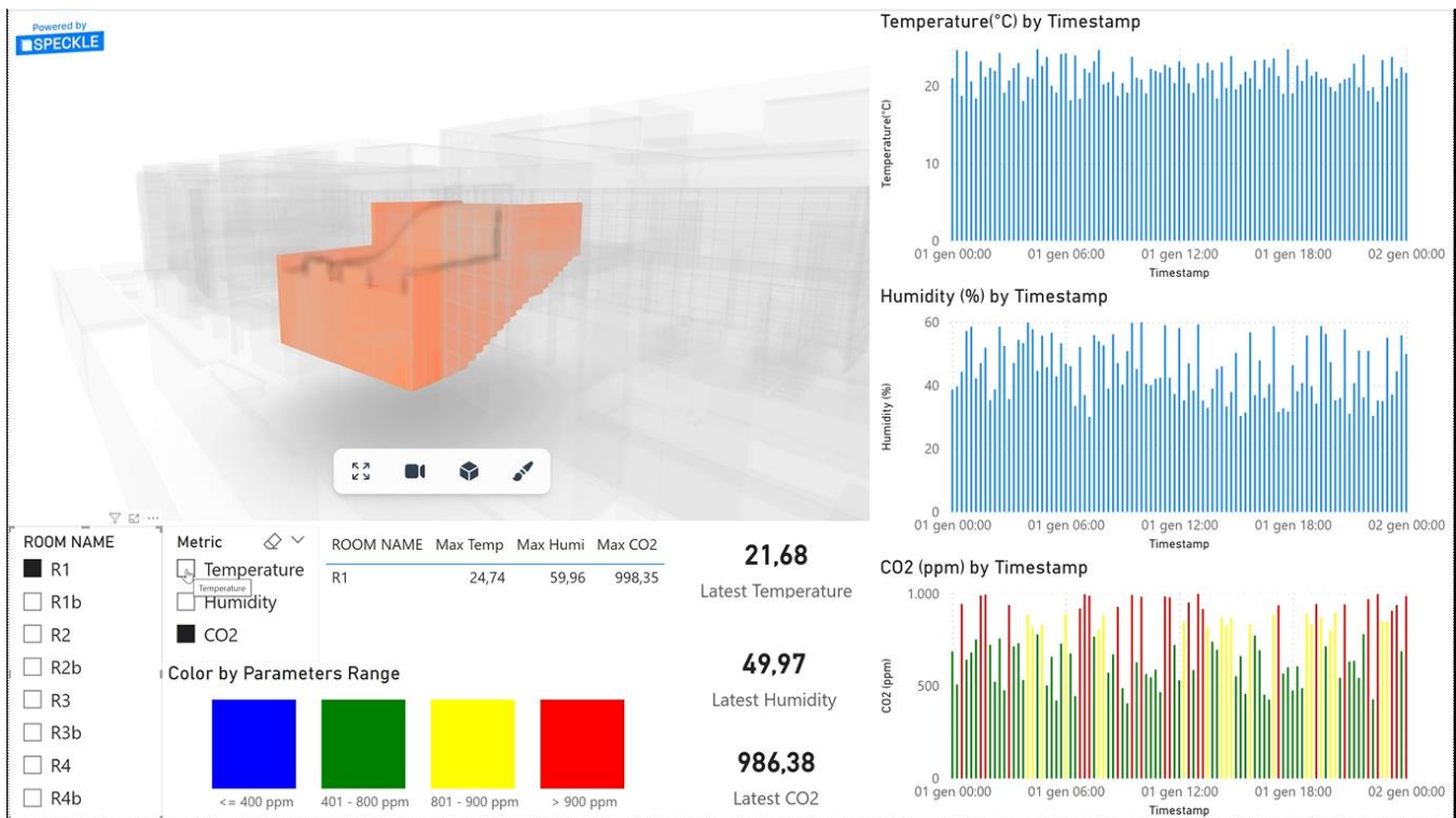
Figure 4.39 BIM-Power BI dashboard developed during internship, visualizing historical data across the 3D model of Aule R.
