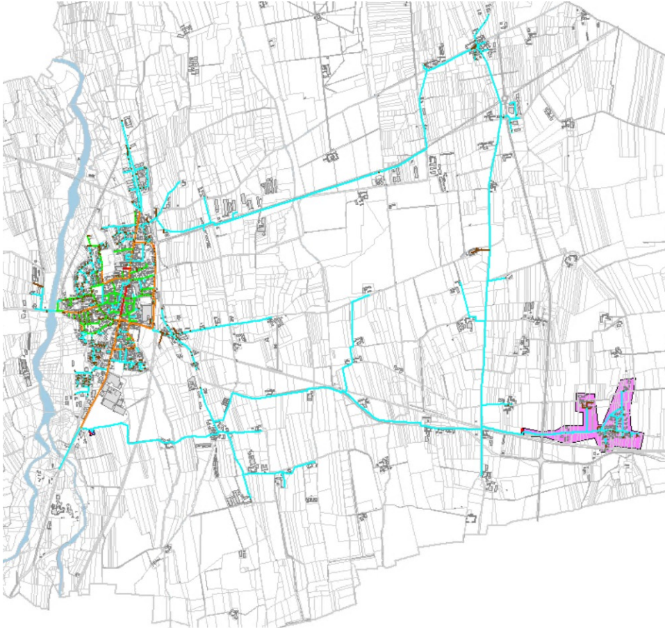
Figure 3.3: GIS Master representation of the Cavallermaggiore water distribution network showing pipes, nodes, tanks, and pumps extracted from the utility database.
