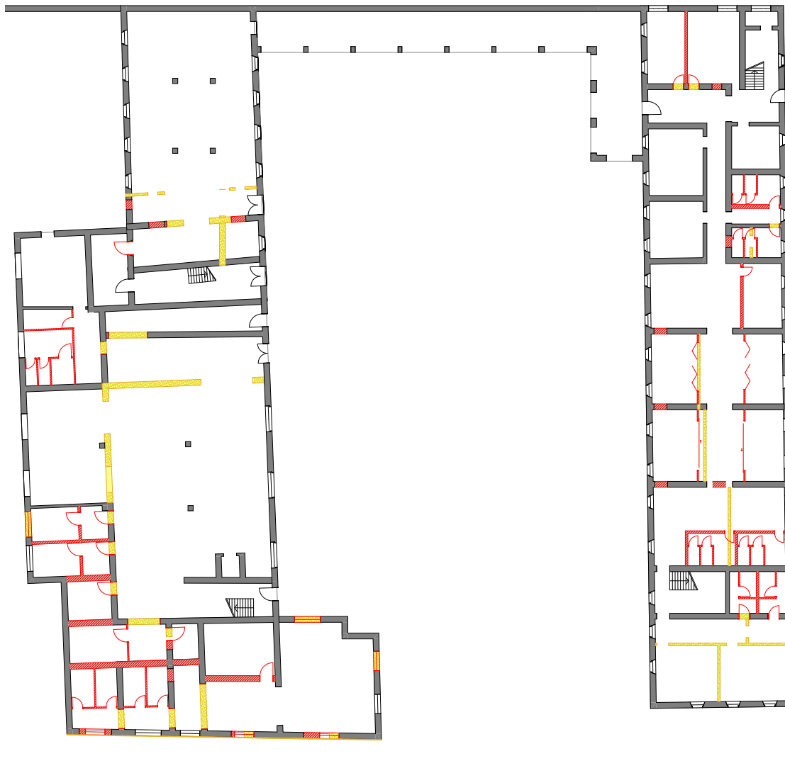
fig.70 Ground floor plan of Sisters' House I,II, Laundry room, demolition - construction.
