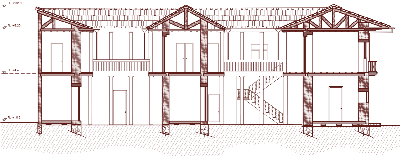
section cut d-d' (sc 1:200)
